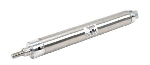
NITRA pneumatic cylinder, non-repairable, 1-1/2in bore, 7/16in rod diameter, 9in stroke, double acting, magnetic piston, rear pivot mount.
