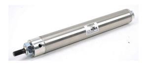
NITRA pneumatic cylinder, non-repairable, 1-1/2in bore, 7/16in rod diameter, 9in stroke, double acting, front nose mount.
