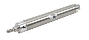
NITRA pneumatic cylinder, non-repairable, 1-1/2in bore, 7/16in rod diameter, 8in stroke, double acting, magnetic piston, rear pivot mount.
