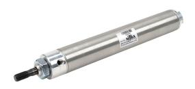
NITRA pneumatic cylinder, non-repairable, 1-1/2in bore, 7/16in rod diameter, 8in stroke, double acting, front nose mount.
