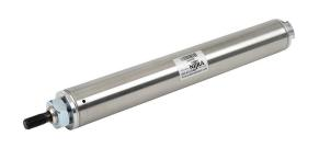
NITRA pneumatic cylinder, non-repairable, 1-1/2in bore, 7/16in rod diameter, 6in stroke, single acting, front nose mount.
