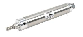
NITRA pneumatic cylinder, non-repairable, 1-1/2in bore, 7/16in rod diameter, 6in stroke, double acting, magnetic piston, rear pivot mount.
