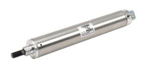
NITRA pneumatic cylinder, non-repairable, 1-1/2in bore, 7/16in rod diameter, 5in stroke, single acting, rear pivot mount.
