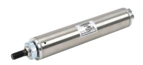
NITRA pneumatic cylinder, non-repairable, 1-1/2in bore, 7/16in rod diameter, 4in stroke, single acting, front nose mount.
