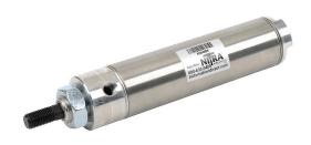
NITRA pneumatic cylinder, non-repairable, 1-1/2in bore, 7/16in rod diameter, 4in stroke, double acting, front nose mount.
