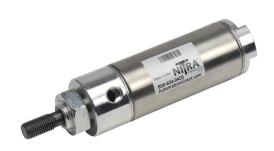
NITRA pneumatic cylinder, non-repairable, 1-1/2in bore, 7/16in rod diameter, 3in stroke, double acting, front nose mount.
