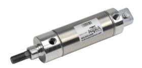
NITRA pneumatic cylinder, non-repairable, 1-1/2in bore, 7/16in rod diameter, 2in stroke, double acting, rear pivot mount.
