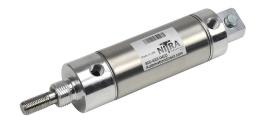
NITRA pneumatic cylinder, non-repairable, 1-1/2in bore, 7/16in rod diameter, 2in stroke, double acting, magnetic piston, rear pivot mount.
