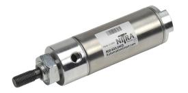
NITRA pneumatic cylinder, non-repairable, 1-1/2in bore, 7/16in rod diameter, 2in stroke, double acting, front nose mount.
