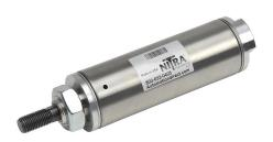
NITRA pneumatic cylinder, non-repairable, 1-1/2in bore, 7/16in rod diameter, 1in stroke, single acting, front nose mount.
