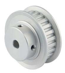
Sung-II Machinery timing pulley, aluminum, 1/5in XL pitch, 24 tooth, 1.528in pitch diameter, 1/4in bore, hub with flanges. For use with 3/8in wide belt.
