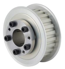
Sung-Il Machinery timing pulley, aluminum, 3/8in L pitch, 24 tooth, 2.865in pitch diameter, 1in bore, no hub with flanges. For use with 1in wide belt. QD bushing included.
