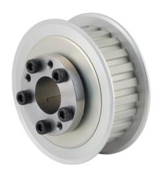
Sung-Il Machinery timing pulley, aluminum, 3/8in L pitch, 24 tooth, 2.865in pitch diameter, 7/8in bore, no hub with flanges. For use with 1in wide belt. QD bushing included.
