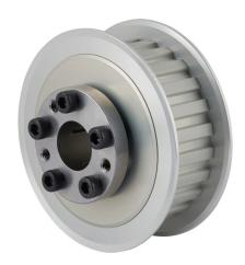
Sung-Il Machinery timing pulley, aluminum, 3/8in L pitch, 24 tooth, 2.865in pitch diameter, 3/4in bore, no hub with flanges. For use with 1in wide belt. QD bushing included.
