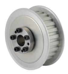
Sung-Il Machinery timing pulley, aluminum, 3/8in L pitch, 24 tooth, 2.865in pitch diameter, 5/8in bore, no hub with flanges. For use with 1in wide belt. QD bushing included.
