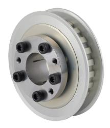
Sung-Il Machinery timing pulley, aluminum, 3/8in L pitch, 24 tooth, 2.865in pitch diameter, 1in bore, no hub with flanges. For use with 1/2in wide belt. QD bushing included.
