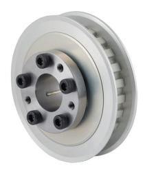
Sung-Il Machinery timing pulley, aluminum, 3/8in L pitch, 24 tooth, 2.865in pitch diameter, 7/8in bore, no hub with flanges. For use with 1/2in wide belt. QD bushing included.
