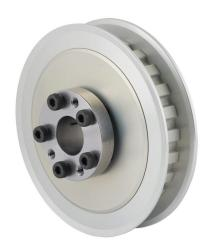
Sung-Il Machinery timing pulley, aluminum, 3/8in L pitch, 24 tooth, 2.865in pitch diameter, 5/8in bore, no hub with flanges. For use with 1/2in wide belt. QD bushing included.
