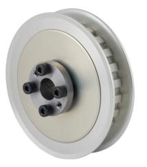
Sung-Il Machinery timing pulley, aluminum, 3/8in L pitch, 24 tooth, 2.865in pitch diameter, 1/2in bore, no hub with flanges. For use with 1/2in wide belt. QD bushing included.
