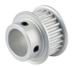
Sung-Il Machinery timing pulley, aluminum, 5mm 5M pitch, 24 tooth, 1.504in pitch diameter, 7/8in bore, hub with flanges. For use with 15mm wide belt.
