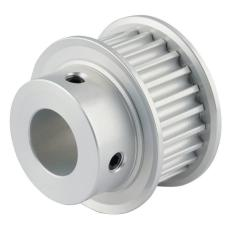
Sung-Il Machinery timing pulley, aluminum, 5mm 5M pitch, 24 tooth, 1.504in pitch diameter, 5/8in bore, hub with flanges. For use with 15mm wide belt.
