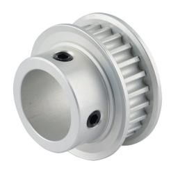
Sung-Il Machinery timing pulley, aluminum, 5mm 5M pitch, 24 tooth, 1.504in pitch diameter, 7/8in bore, hub with flanges. For use with 9mm wide belt.
