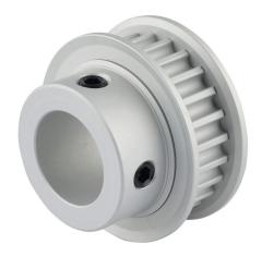
Sung-II Machinery timing pulley, aluminum, 5mm 5M pitch, 24 tooth, 1.504in pitch diameter, 3/4in bore, hub with flanges. For use with 9mm wide belt.
