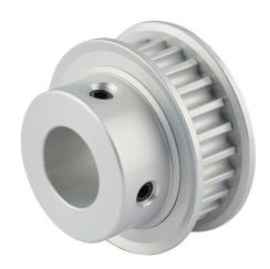
Sung-Il Machinery timing pulley, aluminum, 5mm 5M pitch, 24 tooth, 1.504in pitch diameter, 5/8in bore, hub with flanges. For use with 9mm wide belt.
