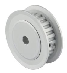
Sung-Il Machinery timing pulley, aluminum, 1/5in XL pitch, 22 tooth, 1.401in pitch diameter, 1/4in bore, no hub with flanges. For use with 3/8in wide belt.
