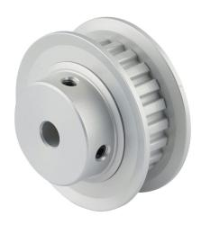
Sung-II Machinery timing pulley, aluminum, 1/5in XL pitch, 22 tooth, 1.401in pitch diameter, 1/4in bore, hub with flanges. For use with 3/8in wide belt.
