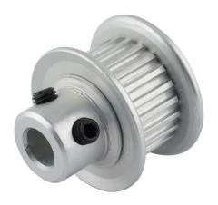
Sung-II Machinery timing pulley, aluminum, 0.08in MXL pitch, 22 tooth, 0.56in pitch diameter, 3/16in bore, hub with flanges. For use with 1/4in wide belt.
