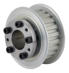
Sung-Il Machinery timing pulley, aluminum, 3/8in L pitch, 22 tooth, 2.626in pitch diameter, 1in bore, no hub with flanges. For use with 1in wide belt. QD bushing included.
