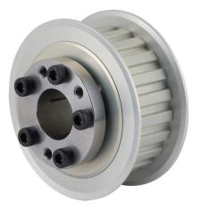
Sung-Il Machinery timing pulley, aluminum, 3/8in L pitch, 22 tooth, 2.626in pitch diameter, 7/8in bore, no hub with flanges. For use with 1in wide belt. QD bushing included.
