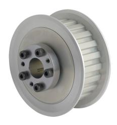
Sung-Il Machinery timing pulley, aluminum, 3/8in L pitch, 22 tooth, 2.626in pitch diameter, 5/8in bore, no hub with flanges. For use with 1in wide belt. QD bushing included.
