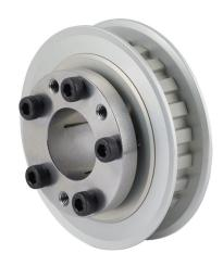
Sung-Il Machinery timing pulley, aluminum, 3/8in L pitch, 22 tooth, 2.626in pitch diameter, 1in bore, no hub with flanges. For use with 1/2in wide belt. QD bushing included.
