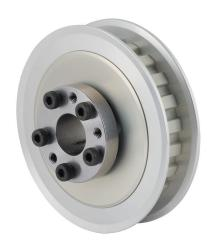
Sung-Il Machinery timing pulley, aluminum, 3/8in L pitch, 22 tooth, 2.626in pitch diameter, 5/8in bore, no hub with flanges. For use with 1/2in wide belt. QD bushing included.
