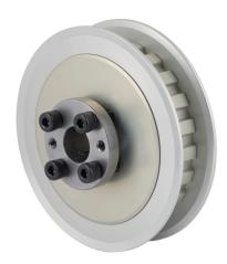
Sung-Il Machinery timing pulley, aluminum, 3/8in L pitch, 22 tooth, 2.626in pitch diameter, 1/2in bore, no hub with flanges. For use with 1/2in wide belt. QD bushing included.
