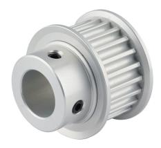
Sung-Il Machinery timing pulley, aluminum, 5mm 5M pitch, 22 tooth, 1.379in pitch diameter, 5/8in bore, hub with flanges. For use with 15mm wide belt.
