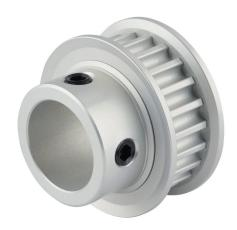
Sung-Il Machinery timing pulley, aluminum, 5mm 5M pitch, 22 tooth, 1.379in pitch diameter, 3/4in bore, hub with flanges. For use with 9mm wide belt.
