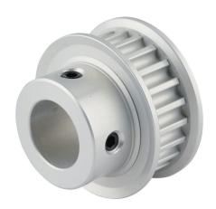
Sung-II Machinery timing pulley, aluminum, 5mm 5M pitch, 22 tooth, 1.379in pitch diameter, 5/8in bore, hub with flanges. For use with 9mm wide belt.
