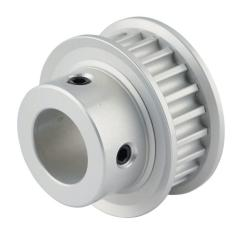
Sung-Il Machinery timing pulley, aluminum, 5mm 5M pitch, 22 tooth, 1.379in pitch diameter, 5/8in bore, hub with flanges. For use with 9mm wide belt.
