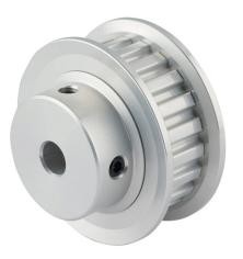
Sung-Il Machinery timing pulley, aluminum, 1/5in XL pitch, 21 tooth, 1.337in pitch diameter, 1/4in bore, hub with flanges. For use with 3/8in wide belt.
