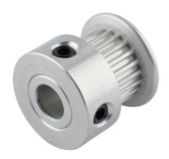
Sung-Il Machinery timing pulley, aluminum, 0.08in MXL pitch, 21 tooth, 0.535in pitch diameter, 1/4in bore, oversize hub with flange. For use with 1/4in wide belt.
