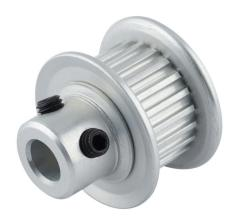
Sung-Il Machinery timing pulley, aluminum, 0.08in MXL pitch, 21 tooth, 0.535in pitch diameter, 3/16in bore, hub with flanges. For use with 1/4in wide belt.
