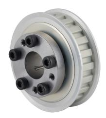
Sung-Il Machinery timing pulley, aluminum, 3/8in L pitch, 21 tooth, 2.507in pitch diameter, 3/4in bore, no hub with flanges. For use with 1/2in wide belt. QD bushing included.
