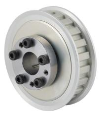
Sung-Il Machinery timing pulley, aluminum, 3/8in L pitch, 21 tooth, 2.507in pitch diameter, 5/8in bore, no hub with flanges. For use with 1/2in wide belt. QD bushing included.
