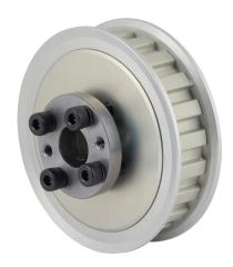
Sung-Il Machinery timing pulley, aluminum, 3/8in L pitch, 21 tooth, 2.507in pitch diameter, 1/2in bore, no hub with flanges. For use with 1/2in wide belt. QD bushing included.
