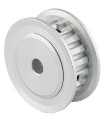
Sung-Il Machinery timing pulley, aluminum, 1/5in XL pitch, 20 tooth, 1.273in pitch diameter, 1/4in bore, no hub with flanges. For use with 3/8in wide belt.
