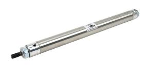
NITRA pneumatic cylinder, non-repairable, 1-1/4in bore, 7/16in rod diameter, 12in stroke, double acting, double end mount.
