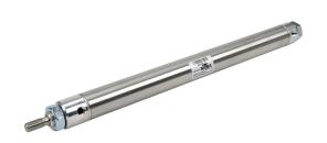
NITRA pneumatic cylinder, non-repairable, 1-1/4in bore, 7/16in rod diameter, 12in stroke, double acting, magnetic piston, double end mount.
