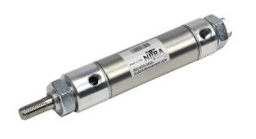
NITRA pneumatic cylinder, non-repairable, 1-1/4in bore, 7/16in rod diameter, 10in stroke, double acting, double end mount.
